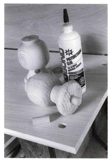
Use 3/4/" dowel and one of the new polyurethane glues to fasten the feet to the kicker.
